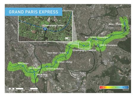
With 200 km of underground metro lines, the GPE is the world's largest project to monitor the impact of tunneling operations on existing surface structures along the alignment and adjacent areas using SqueeSAR $^{\circ}$ .
