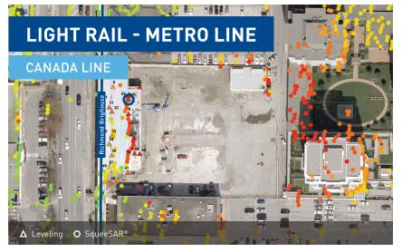
A seven-year satellite monitoring over the rapid transit system linking Vancouver downtown to the airport and the city of Richmond, to detect ground instabilities along the line. The image refers to the Brighouse station area during construction.
