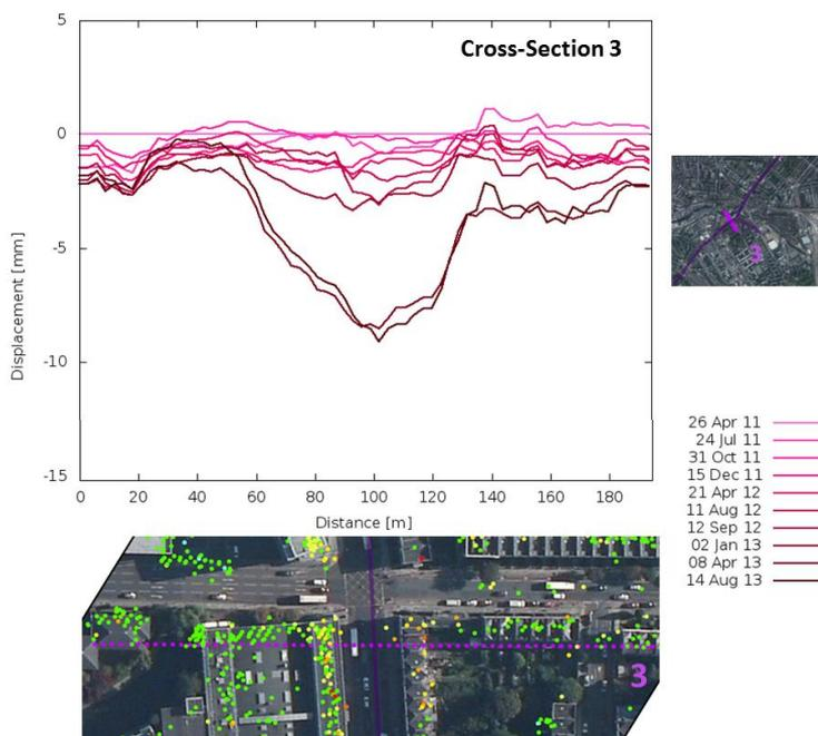
**Fig. 2** CS3 shows the sudden increase of motion between January and April 2013 and its subsequent stabilization after that period
