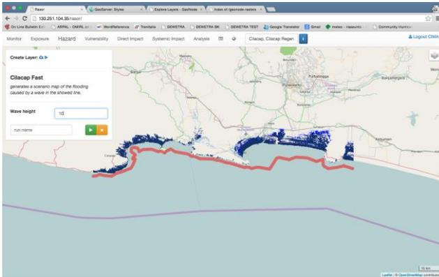
Figure 6. The *Hazard* module - Interface of tsunami module over Cilacap (Indonesia).
