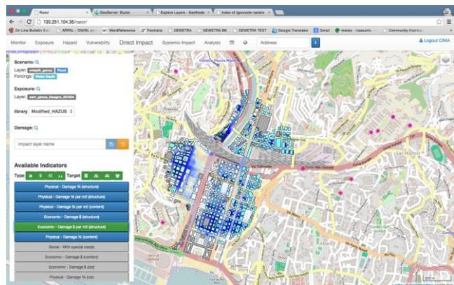
Figure 8. The *Impacts* module - Example of economic damage computation for buildings in the city of Genoa.
