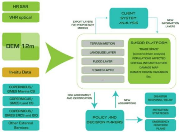
Figure 2. RASOR platform architecture.
