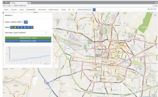
Figure 7. The *Vulnerability* module - The assets can be evaluated and mapped with respect to their degree of vulnerability characterization.
