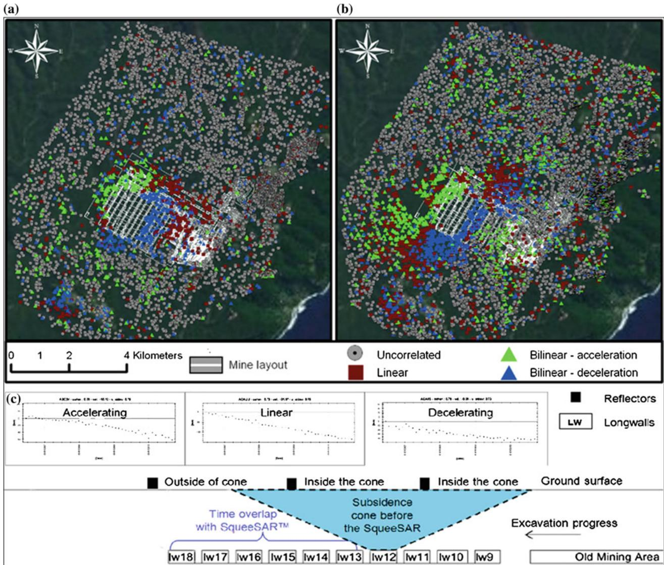
**Fig. 187.2** Results of the time series classification with PS-Time of **a** Descending dataset and **b** Ascending dataset. Both geometries show a clear localization of measurement points showing acceleration (front of the mine excavation direction) while measurement points showing deceleration are located at the back of the mine layout, over old
