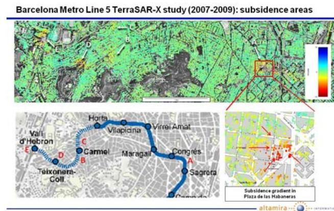
Figure 1. Movement evolution in Barcelona city because of Metro construction (2007-2009)
