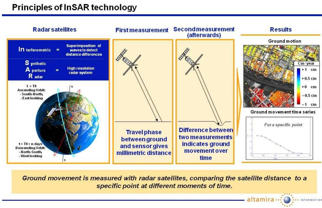
Figure 1 Basic principles of radar interferometry.
