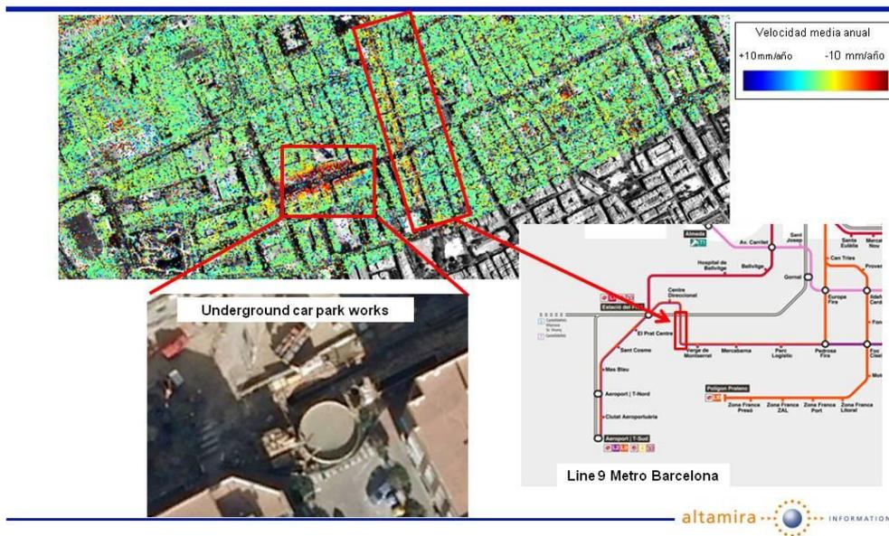
Figure 4 Surface movement due to the construction of a car park and Metro Line 9 (Barcelona)
