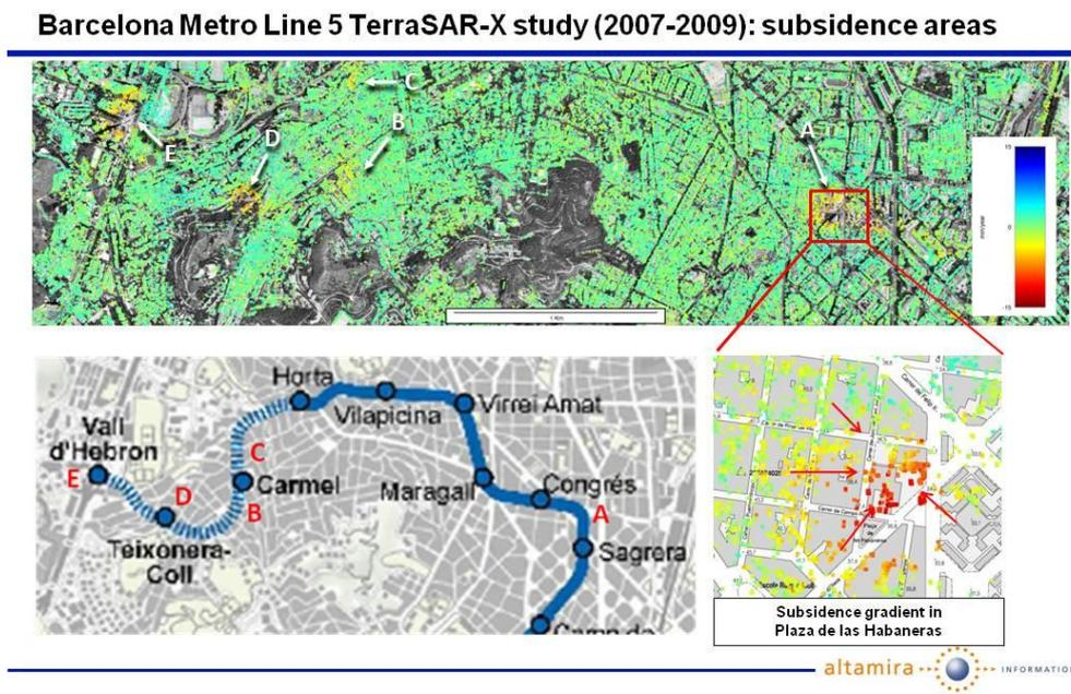
Figure 2 Movement evolution in Barcelona city because of Metro construction (2007-2009)
