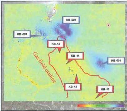
Figure 2 Example for subsidence map produced from SqueeSAR.
