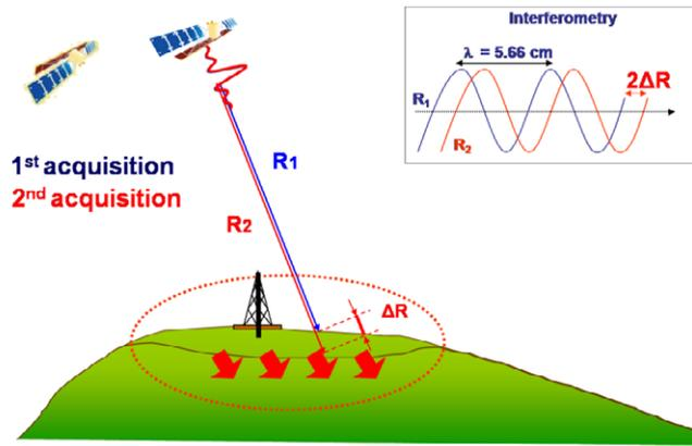
Figure 1: A schematic showing the relationship between ground displacement and signal phase shift. The numeric value of the wavelength  $\lambda$  is that used by the ERS satellite operated by the European Space Agency (ESA).
