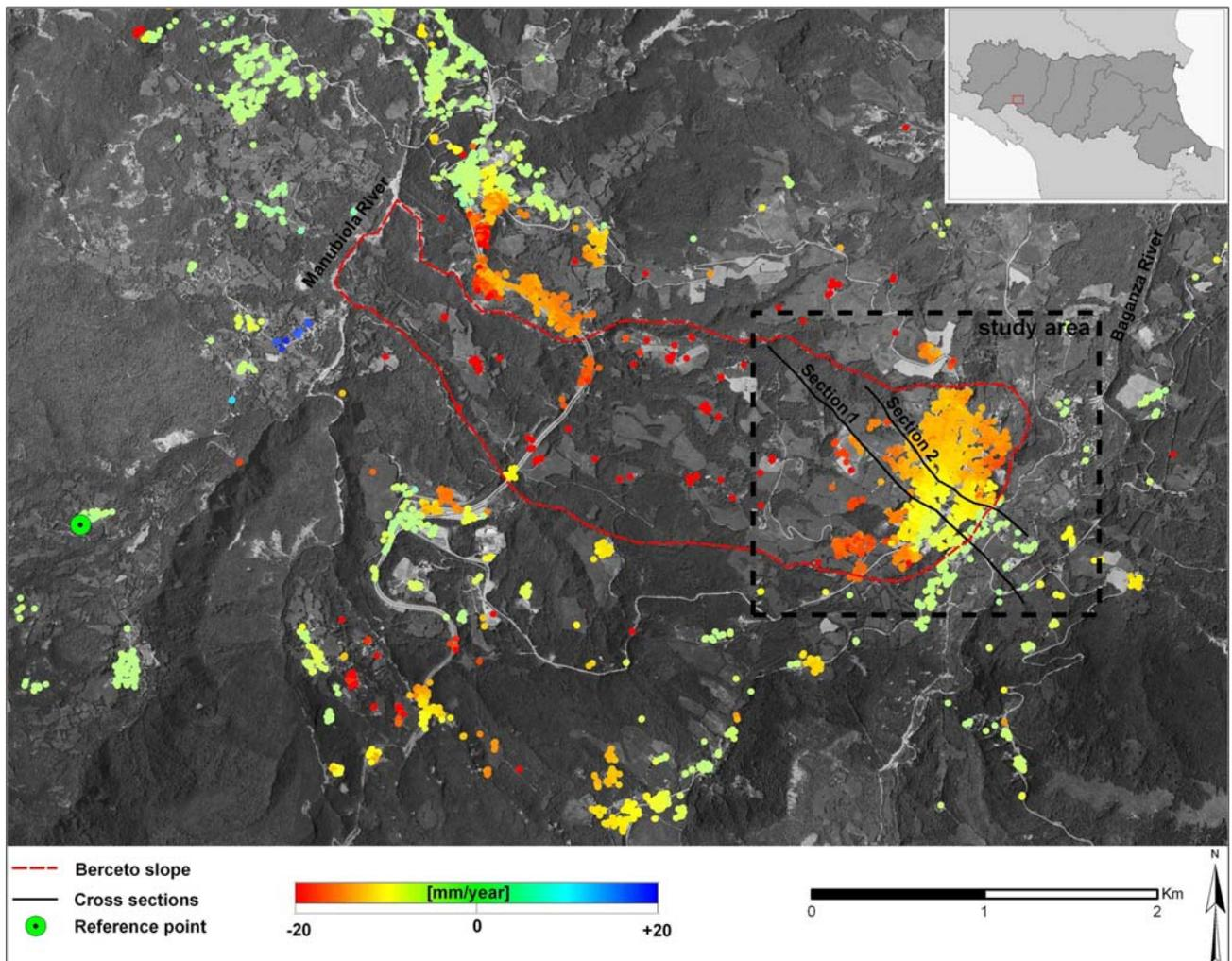
Figure 1 Location map of the study area, with the average yearly surface displacement velocity measured along the satellite LOS.
