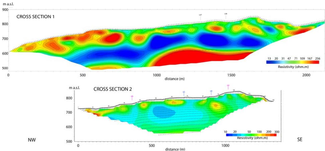
Figure 5 DC resistivity tomography profiles 1 (by GEOINVEST s.r.l. Piacenza, up) and 2 (by SGG s.r.l. Siena, down).
