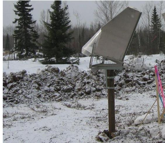
Fig. 7: Artificial Corner Reflectors
