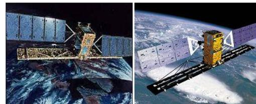
Fig. 2: Radar satellites owned by the Canadian Space Agency (CSA): Radarsat-1 launched in 1995 and Radarsat-2 launched in 2007
