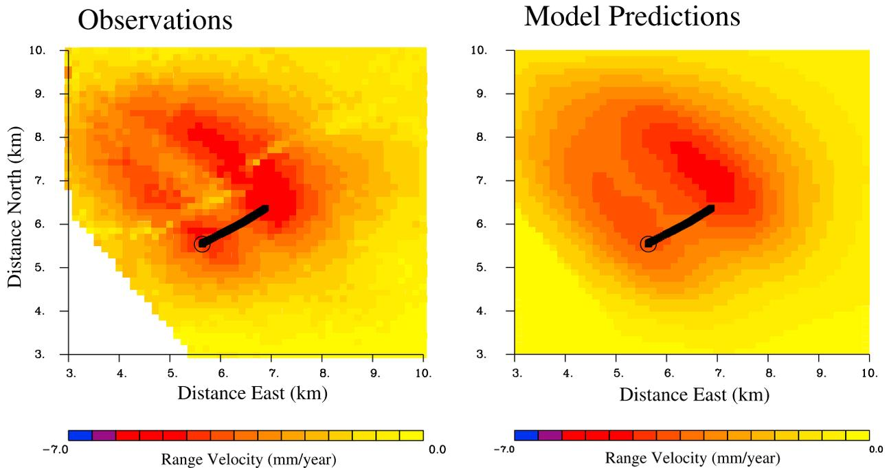
**Figure 4.** (a) Observed range velocities for the permanent scatterers surrounding well KB-502. The data in the lower left corner of the plot were influenced by fluid injection at well KB-503 and hence were not used in the inversion (thus left blank). (b) Range velocities calculated using the model shown in Figure 3 and Wang *et al.*'s [2006] forward modeling approach.
