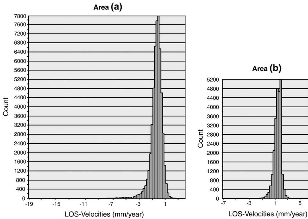
Fig. 3. Histograms of the PSInSAR velocities distribution in the Adige (a) and Sarca (b) valley areas as defined in Fig. 2.
