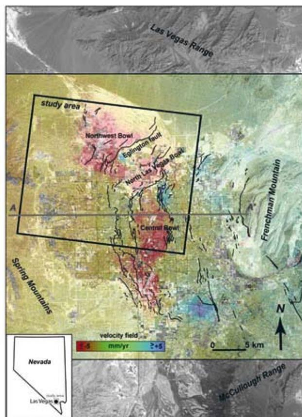
**Figure 2** Permanent scatterer velocity map of a 40 x 40 km framework area in Las Vegas Valley for the period 1996–2000 showing generalized PS rates; red areas denote subsidence and blue areas, uplift. Total number of PS targets in the framework area is more than 500,000. Study area (inset box) is a smaller subset (90,000 targets) of the PS data covering the northwest part of the valley.
