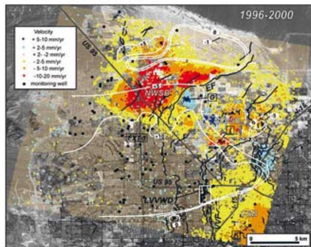
**Figure 4b** Permanent scatterer velocity map from ERS data for the period 18 April 1996 to 28 April 2000 and water-level change for the period April 1996 to May 2000.
