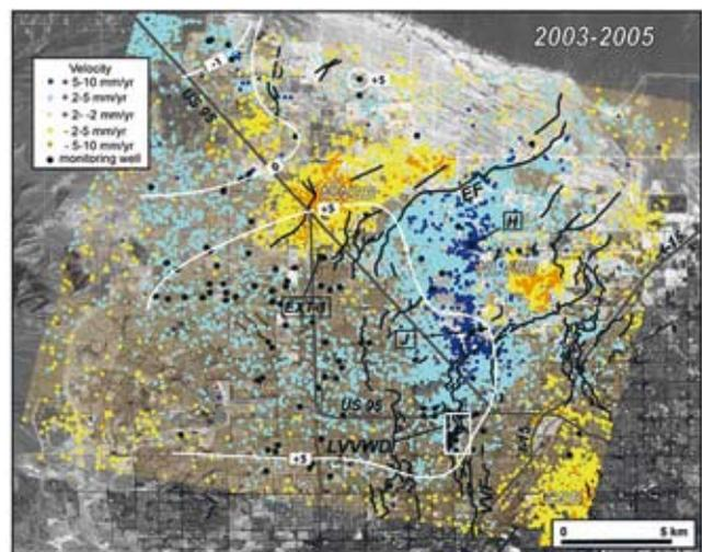
**Figure 4c** Permanent scatterer velocity map from ENVISAT data for the period 18 April 2003 to 27 May 2005 and water-level change for the period April 2003 to May 2005.
