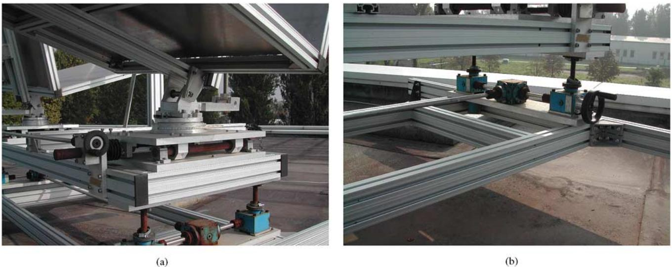
Fig. 2. Mobile reflectors' assembly. The (a) vertical and (b) horizontal translation mechanism.
