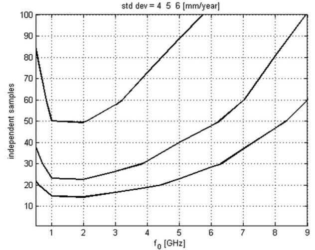
Fig. 11. Number of pixels equivalent to a PS as a function of frequency for various velocity dispersions (4, 5, and 6 mm/year; 12 days repeat).
