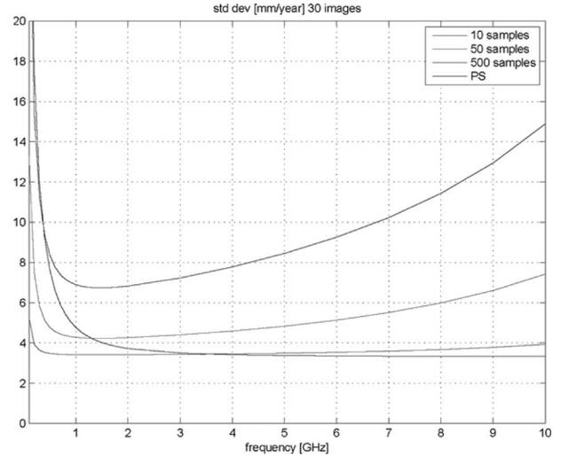
Fig. 10. Dispersion of the estimate of the subsidence rate is shown as a function of frequency for different values of the number of looks ( $L = 10, 50, 500$  and  $N = 30$ ) and for a PS.
