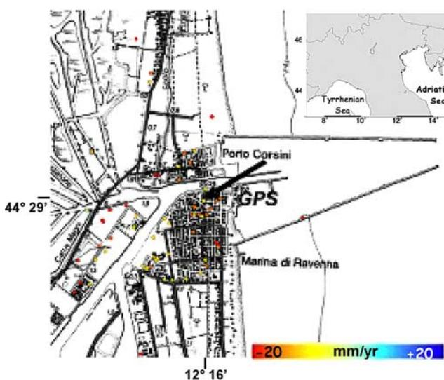
**Figure 7.** Distribution of PSs in the Marina di Ravenna area, relevant subsidence rates, and location of the GPS station. The location of the SAR images is shown in the right upper corner.
