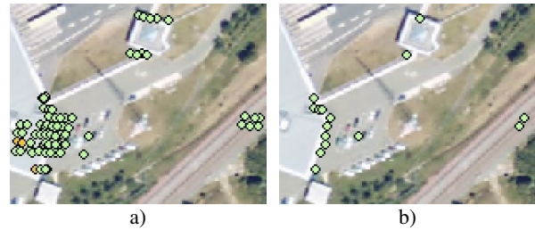
Figure 9. Example final geocoded SPN mean rate subsidence. a) result of a normal geocoded final selection based on the SPN model coherence. b) improved final selection considering only the centre of the main lobe for strong scatterers.
