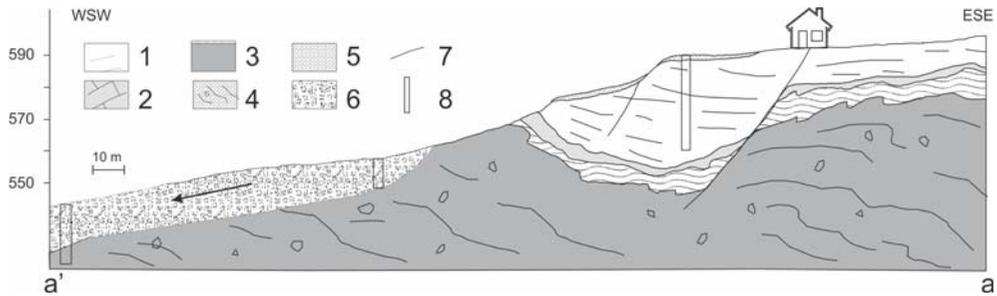
**Fig. 4** Longitudinal section of the depletion zone of the Poggio Ferrato landslide. 1: M. Vallassa Sandstone; 2: Monte Lumello Marls; 3: M. Piano Marls; 4: Chaotic Complex; 5: weathered sandstone; 6: landslide; 7: fracture; 8: borehole.
