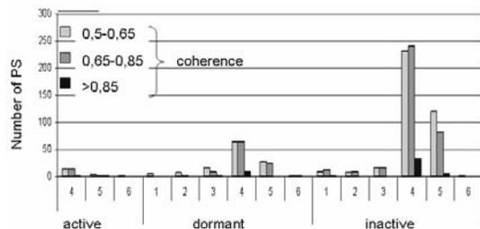
**Fig.2** PS distribution vs landslide activity. Velocity classes 1: < -5 mm/yr, 2: -3/-5 mm/yr, 3: -1/-3 mm/yr, 4: -1/+1 mm/yr; 5: +1/+3 mm/yr; 6: +3/+5 mm/yr; 7: > +5 mm/yr.
