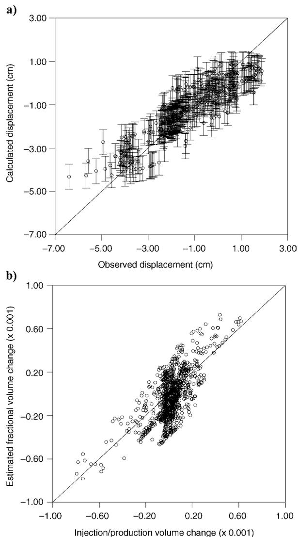
Figure 7. (a) Displacement values, calculated using the volume-change model, which resulted from the inversion. These values are plotted against the observed displacement values. For a perfect fit, the points would plot on the diagonal line shown. The errors bars signify one standard deviation. (b) Volume change obtained from the inversion plotted against the volume change from the roaming-tank model. The values along each axis should be multiplied by the numbers in parentheses.
