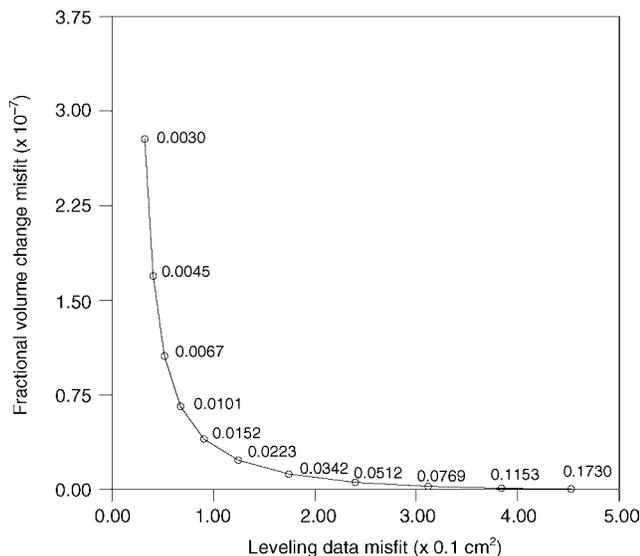
Figure 6. Trade-off curve derived from 11 distinct inversions. The curve represents squared misfit to the leveling data plotted against the squared deviation from the volume changes computed using the roaming-tank model. For each inversion, the norm weighting  $W_n$  in equation 17 was set to the value indicated at each point on the plot. The numerical factors in parentheses indicate the scaling of each axis (i.e., the values along each axis should be multiplied by the numbers in parentheses).
