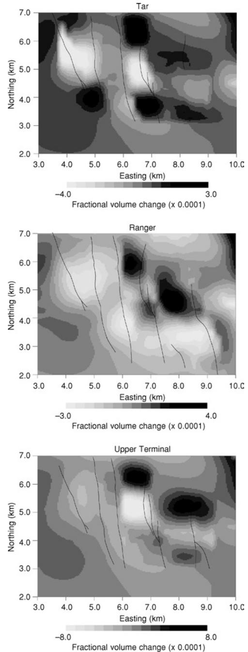
Figure 12. Results of the inversion of the permanent scatterer range-change estimates. Volume change for the three layers in the Wilmington reservoir model. The scale values should be multiplied by the numbers in parentheses.
