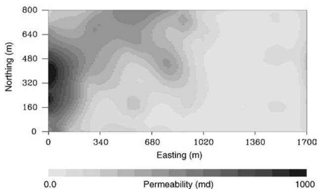
Figure 3. Permeability estimates resulting from an inversion of the surface displacement data.
