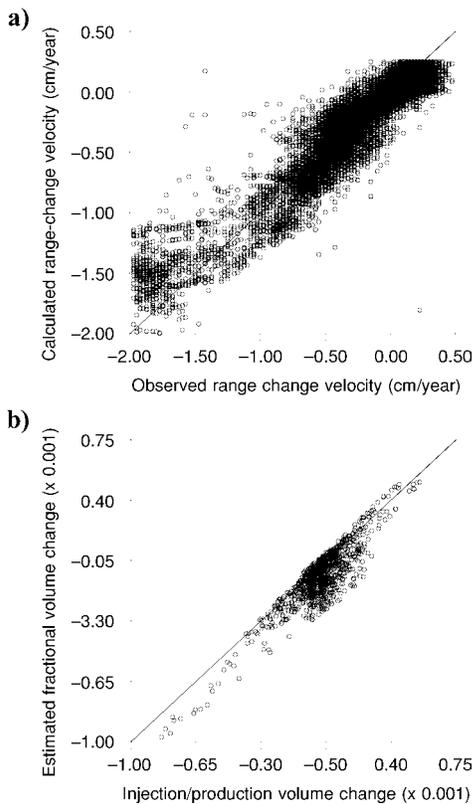
Figure 11. (a) Range-change values, calculated using the volume-change model, which resulted from the inversion. These values are plotted against the observed range changes. (b) Volume change obtained from the inversion, plotted against the volume change from the roaming tank model. The values along each axis should be multiplied by the numbers in parentheses.
