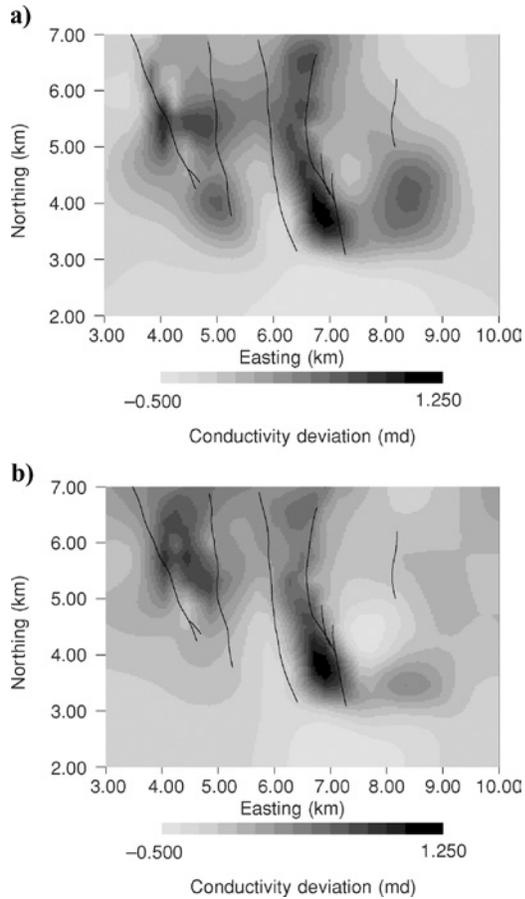
Figure 14. Comparison of permeability estimates made (a) using the permanent scatterer data and (b) based on the leveling data.
