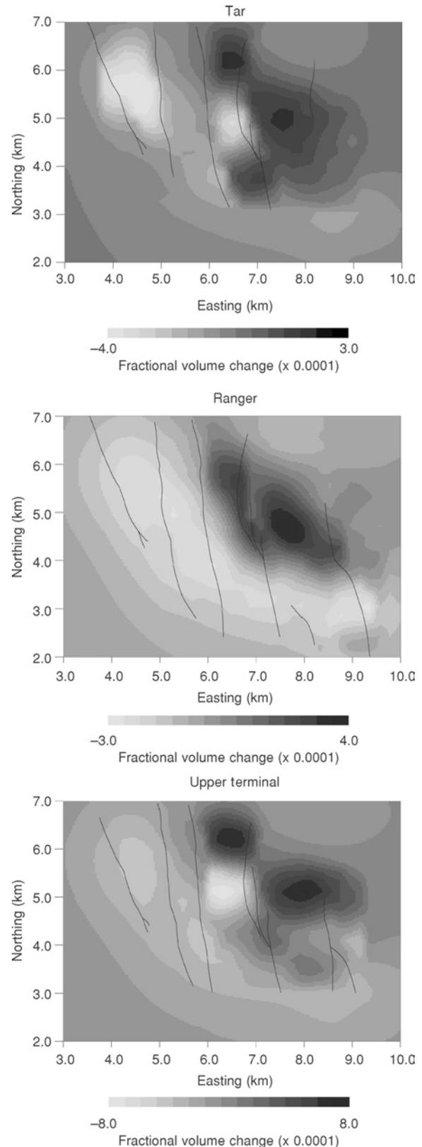
Figure 8. Volume change for the three layers of the Wilmington reservoir model. The solid black lines represent major interpreted faults in each layer. The scale values should be multiplied by the numbers in parentheses.
