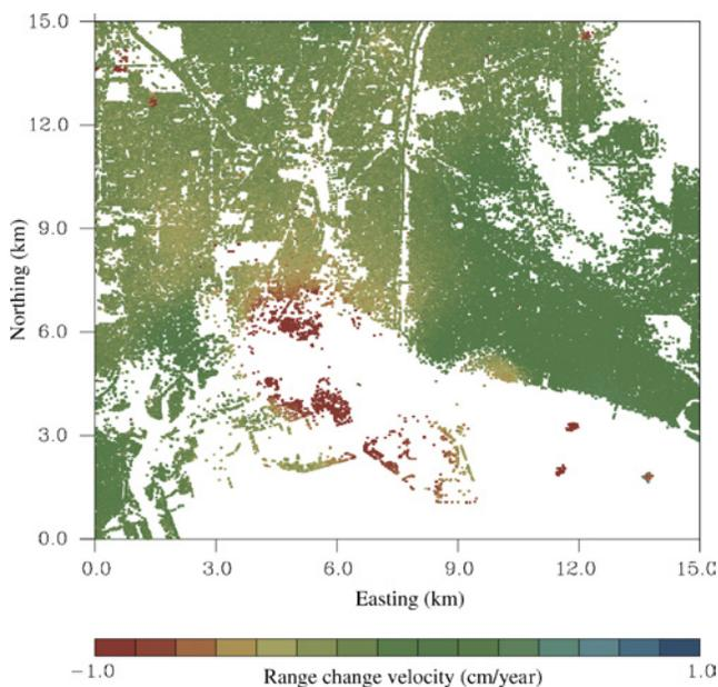
Figure 9. Permanent scatterer estimates of range change over the Long Beach region for the time period June 1992 to June 2000. The white regions indicate pixels for which displacements could not be determined.
