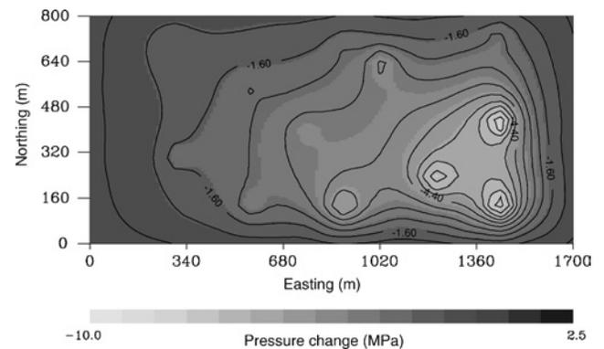
Figure 2. Pressure changes after two years of production from the reservoir model.
