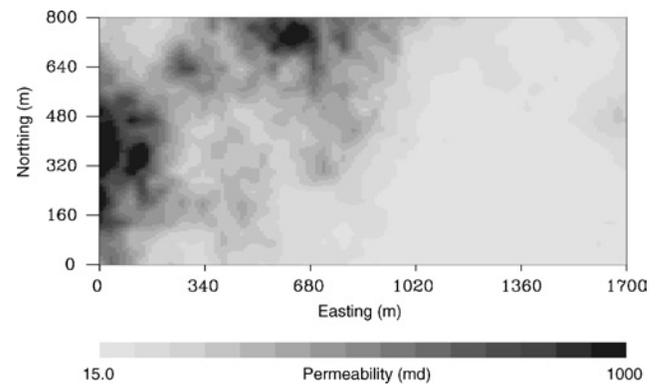
Figure 1. Spatial permeability variation used to generate a set of surface displacement values. The gray scale denotes the permeability variations within the reservoir model.
