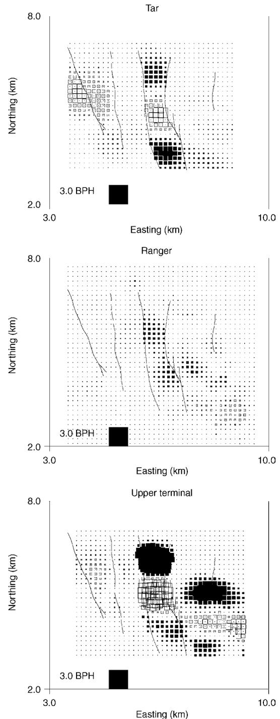
Figure 5. Net volume fluxes into the three main formations of the Wilmington reservoir, calculated using the roaming-tank model. Filled squares denote positive fluid fluxes, whereas open squares indicate withdrawal. The dimensions of each square are proportional to the net volume flux. The reference square represents a net fluid flux of 3.0 barrels per hour.
