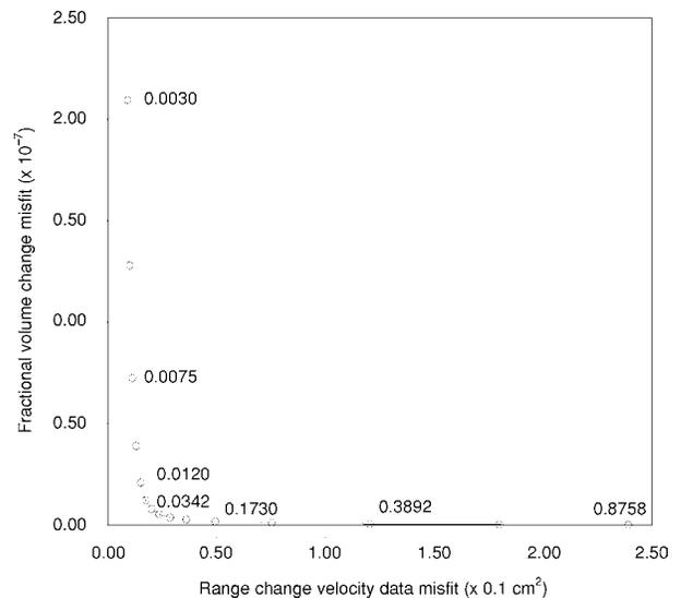
Figure 10. Trade-off curve derived from 15 distinct inversions. This figure is similar to Figure 6. For each inversion, the norm weighting  $W_n$  was set to the value indicated on the plot. The values along each axis should be multiplied by the numbers in parentheses.
