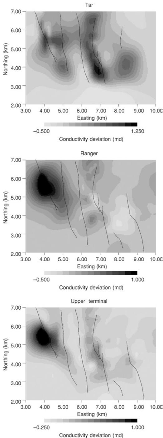
Figure 13. Permeability estimates for the three layers of Wilmington field. The deviations of permeability from an initial uniform model are shown in the figure.
