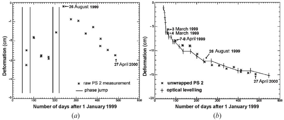
Figure 3. Comparison with optical levelling at PS 2 (after the collapse event of February 1999): (a) ambiguous (phase wrapped) PS measurement; and (b) unwrapped time series of PS 2 compared with the levelling data.
