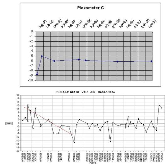
Figure 5. Piezometric and PS readings in the Casalino area.
