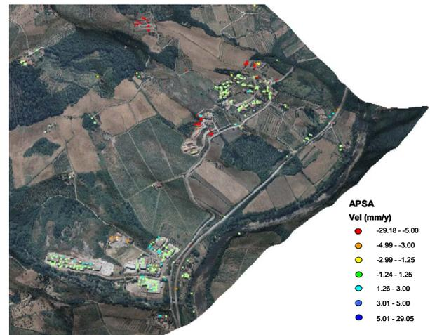
Figure 3. PS of the Carbonile landslide overlaid on an aerial-photo rendered on a 10m cell-size DTM.
