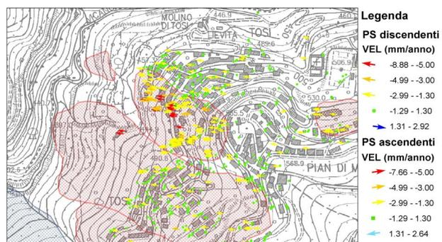
Figure 2. Map overlay of the PS classified with reference to the velocity and the updated landslides inventory map.
