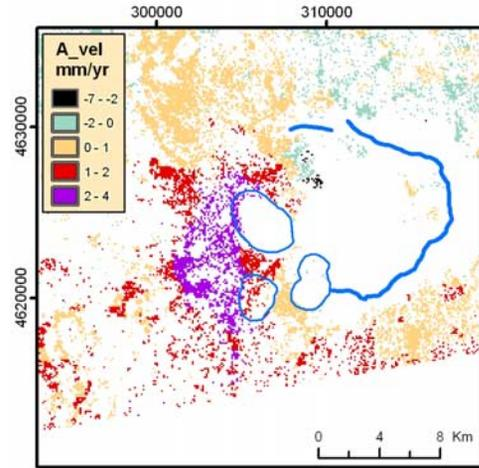
**Figure 3.** Ground velocity in the period 1993–2000, in the ascending ERS orbit. Also shown is the dislocation area for our model 1S. The site of the Solfiorata gas vents is indicated (S).
