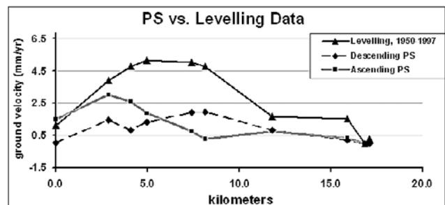
**Figure 4.** Comparison between the ground velocities retrieved by the PS technique in the 1993–2000 period, and the average ground velocity retrieved by leveling in the 1997–1950 period.
