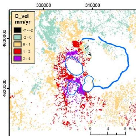
**Figure 2.** Ground velocity in the period 1993–2000, in the Line of Sight of the descending ERS orbit. The site of the Solfiorata gas vents is indicated (S).
