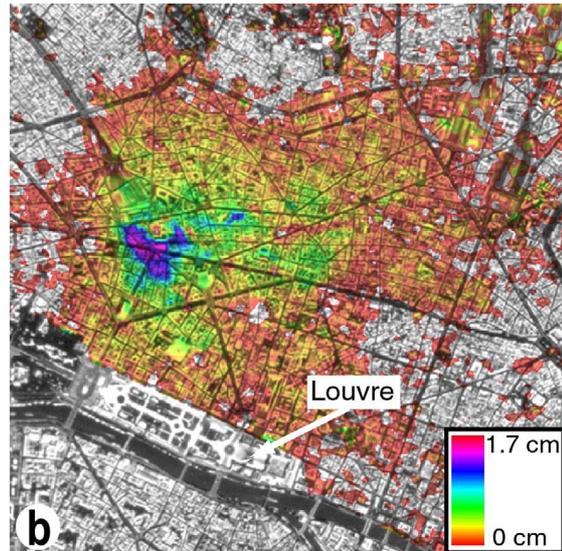
Fig. 4. (b) Map of cumulate uplift due to the end of water pumping and the slow recharge of the nappe (same HIS composition)(processing done by UMLV)
