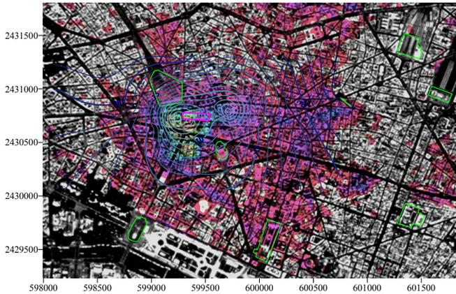
Fig. 5. Superimposition of interferometric and piezometric data for the subsidence
