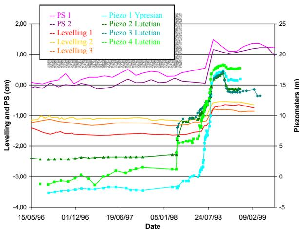
Fig. 6. Comparison between levelling, piezometry and PS .
