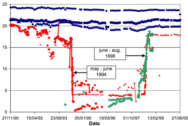
Fig.1. Monitoring of the different aquifers from November 1990 to June 2000). In blue: Alluvium, in red: Lutetian; in green: Ypresian.
