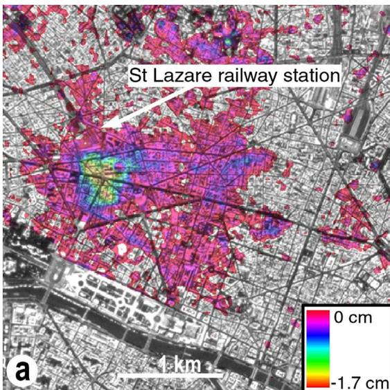
Fig. 4. (a) Map of cumulate subsidence due to the beginning of water pumping: Intensity Hue Saturation composition using an aerial photograph of IGN (©IGN Paris 2001. Poster Paris ISSN BD Ortho®)
