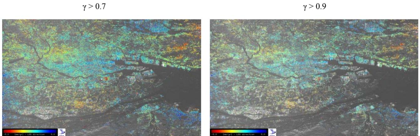
Figure 7: Permanent scatterers in the Noubi plane: left:  $\gamma > .7$ ; 760000PS; right  $\gamma > .9$ ; 240000PS
