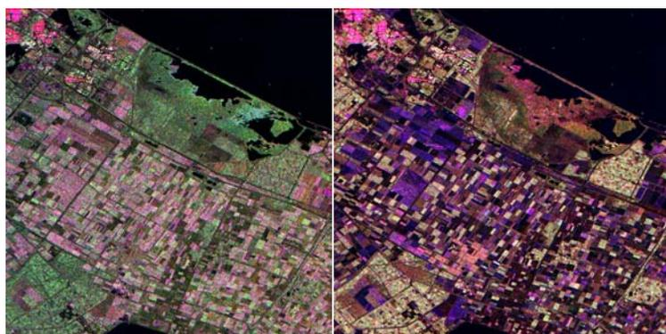
Figure 1: C band and L band (SIR-C/X-SAR images of Flevoland in Holland).
