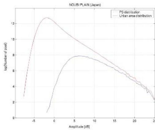
Figure 9: Histograms of amplitudes in an urban area and PS amplitudes: most high amplitude scatterers are PS
