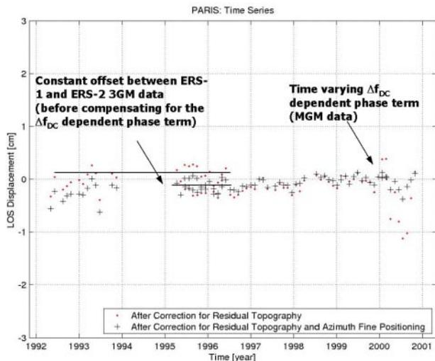
**Figure 1: Displacement time series of a single PS before (red) and after (black) compensating the phase term depending on the sub-cell azimuth PS position coupled with varying (MGM since Feb. 2000) Doppler Centroids. Analogous results have been obtained also involving ZGM ERS-2 data.**
