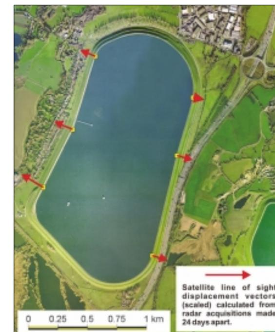
Wraysbury Reservoir with corner reflector sites (Provided courtesy of Nigel Press Associates)
