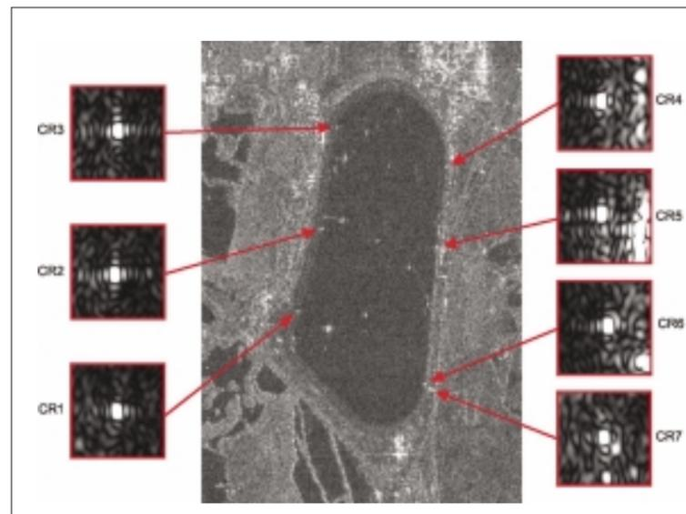
*Satellite Image showing Wraysbury Reservoir with corner reflectors (Provided courtesy of Nigel Press Associates)*
