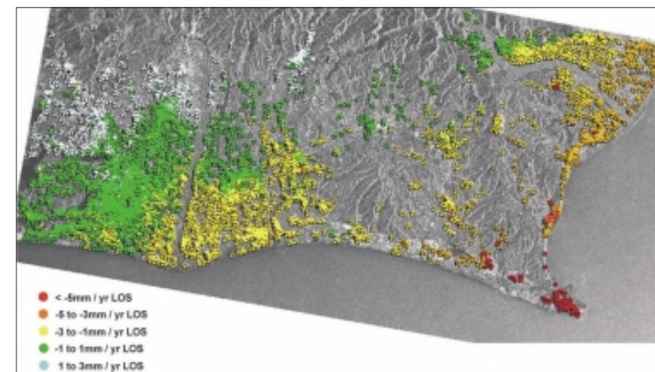
ESA project in Japan (zoomed image): Permanent Scatterer points colour-coded by displacement rate (Provided courtesy of Nigel Press Associates, ImageOne, TRE, GSI, and Willis Reinsurance)
