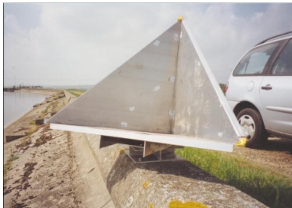
Corner Reflector used in CRInSAR (Provided courtesy of Nigel Press Associates)
