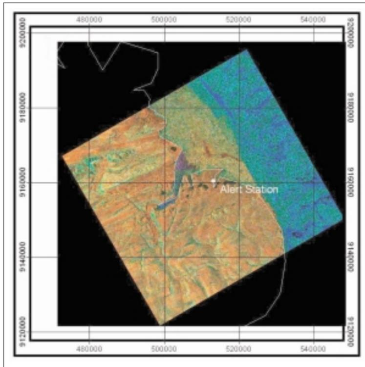
*RADARSAT-1 Digital Elevation Model (DEM) of Alert Bay, NWT Canada displayed in grey scale. Ice velocity displayed in colour scale (+/- 60 cm per month). The estimated height accuracy is 5m, while the horizontal spacing is 10m. (Provided courtesy of Sarmap)*
